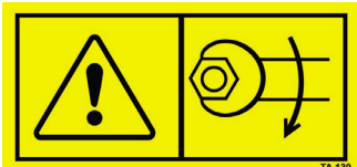
Ensure all nuts & bolts have been tightened prior to operating the machine
