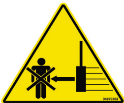
Danger from rotating Prestretcher
