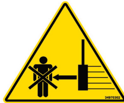
Danger from rotating Pre-stretcher
