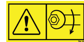
Ensure all nuts & bolts have been tightened prior to operating the machine
