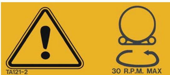
4. DO NOT EXCEED TURNTABLE SPEED OF 30 R.P.M.
